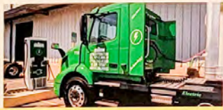
Electric truck charging station
