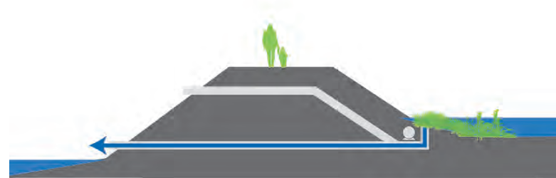
Treatment wetland and levee stormwater management
