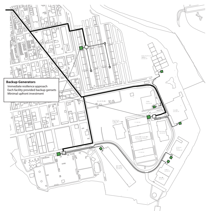
Existing electrical network with diesel backup generators at each facility
